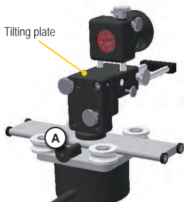
Image showing the prism close to the tilting plate.
