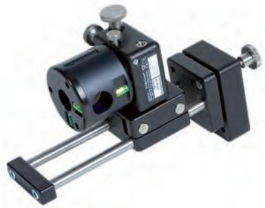
Angular prism D46 is used for parallelism measurement of the flanges. It deflects the laser beam 90°.
