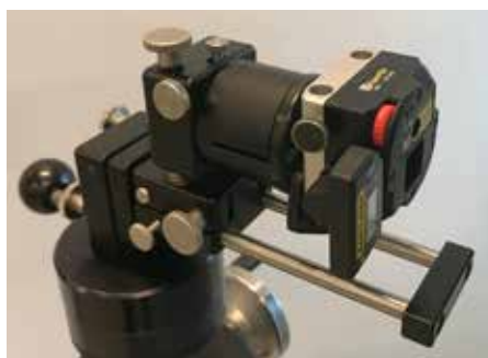
Turn the prism 180° and adjust the offset
