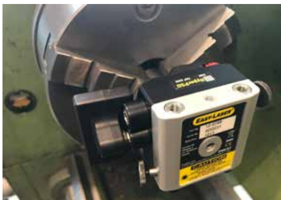
S-unit mounted on the spindle bracket.
