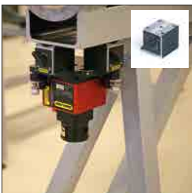
With magnet bases, very rigid mounting.
