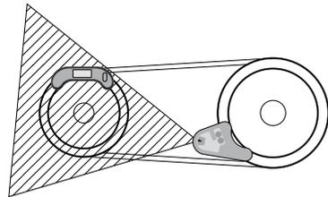
Detector placed for Horizontal alignment. Adjust the Transmitter so that the laser plane hits both the detector apertures.
