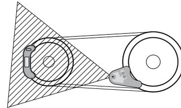
Detector placed for Vertical alignment. Also note Transmitter placement. Adjust the Transmitter so that the laser plane hits both the detector apertures.
