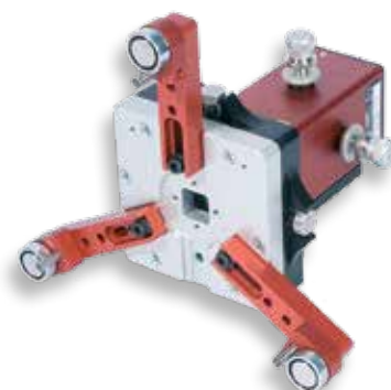
Laser transmitter D75 mounted on a hub
