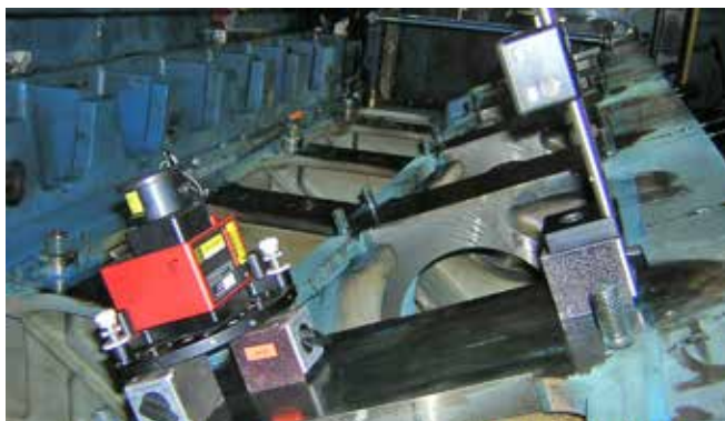
Straightness and flatness on the diesel engine block
