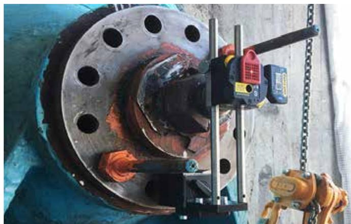
*Measuring unit mounted in the rotational centre. The entire blue section rotates.*
