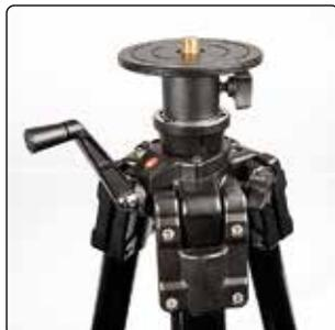
**Tripod****Part No:** 12-0269**Description:** For use with Laser transmitter and Angular prism. Min./Max. height 500–2730 mm [ 19.7–107.5" ]**Note:** Includes tripod head Part No. 03-1338, with 5/8-11 UNC threads.
