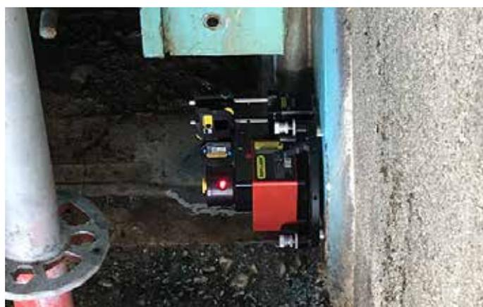
*Laser transmitter D22 mounted with its integrated magnets on the sealing side.*
