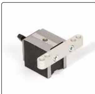
**Small magnet base****Part No:** 12-1092**Description:** To be used when a low and small magnet base is needed. Height 35 mm [1.38"], magnet base width x length appr. 35x30 mm [1.38x1.18"].**Note:** Can be used with D, E and XT series units.
