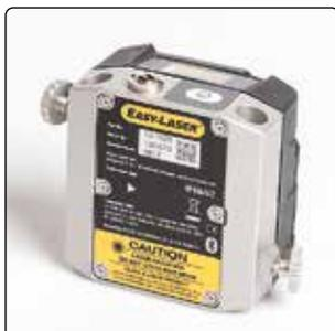
**Measuring unit XT70-M, dot laser, PSD 20x20 mm, 2-axis**
