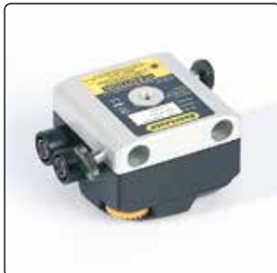
**Measuring unit EMH, dot laser, PSD 20x20 mm**
