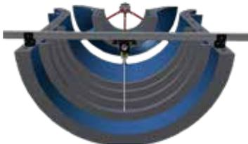
5. Turn detector to 6 o'clock and adjust vertical error to zero.
