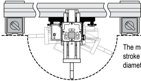
The measuring principle is the same for both long and short stroke bracket. The probe rod is very easily adapted to each diameter with extensions of different length.
