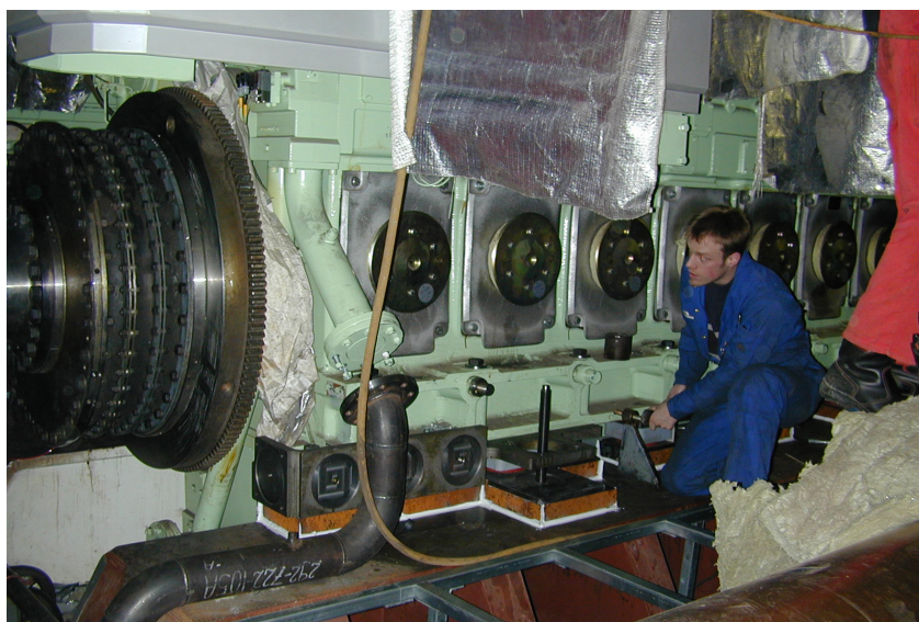
Adjusting the diesel engine
