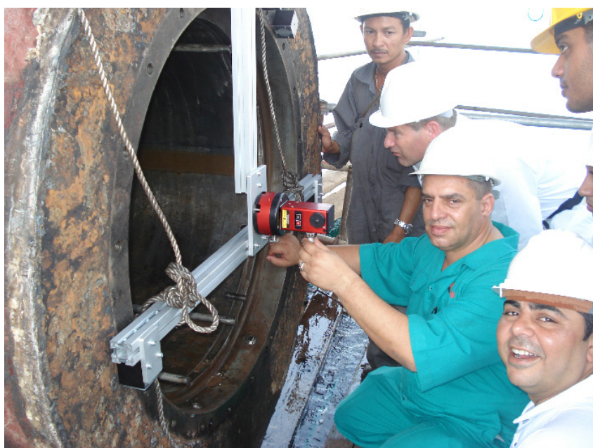
Setting up the laser beam from the sterntube
