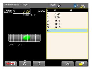
When measuring a shaft using the Precision level, we recommend that the shaft is no larger than 100 mm in diameter.
